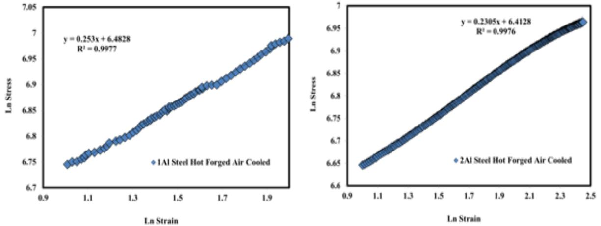
Figure 7: Work-Hardening Coefficient of Both Alloys 1 and 2
