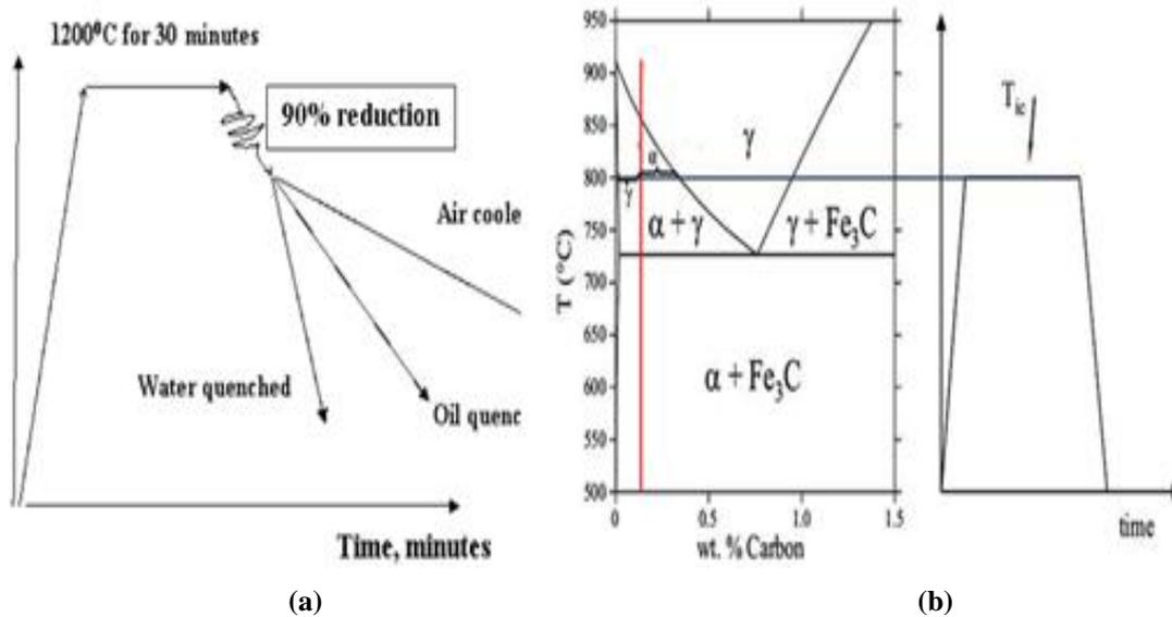
**Figure 1: (a) Thermo-Mechanical Process of Free-Carbide Steel, (b) Intercritical Annealing Process for Dual Phase Steel**
